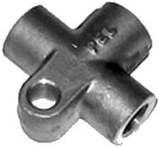
3637/2 RACCORDO A 3 VIE PER TUBI FRENO 500F/L/R GIARD. (BRAKE PIPE CONNECTION)
