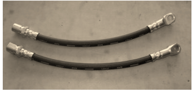
3674 TUBO FRENO ANTERIORE FIAT 500 F/L/R 126 (FRONT BRAKE HOSE)
