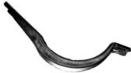
3632 STAFFA MARMITTA 500 F/L INFERIORE LUNGA (BOTTOM MUFFLER BRACKETS FIAT 500 N/D/F/L)
