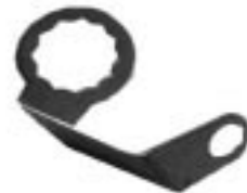
3764 PIASTRINA PER TUBO FRENO ANTERIORE DS. 500/126/600 (FRONT RH FBRAKE HOSE RETAIN PLATE)
