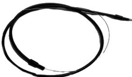
CV018 CAVO APERTURA COFANO ANTERIORE FIAT 500 F/L/R (FRONT HOOD OPENING CABLE)
