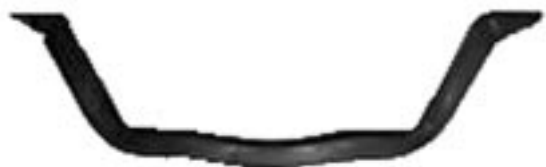
3664 TRAVERSA SUPPORTO CAMBIO FIAT500 N/D/F/L GIARDINIERA (GEAR BOX CROSS RAIL)
